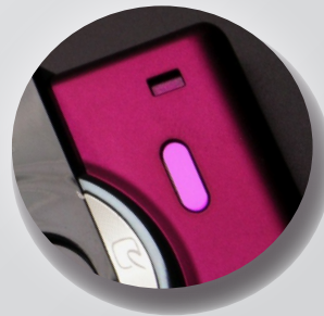
Bordeaux color IR window on IrDA communication port of smart phone
