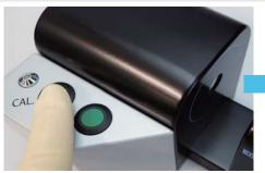
Push the CAL button and then the calibration is performed.
